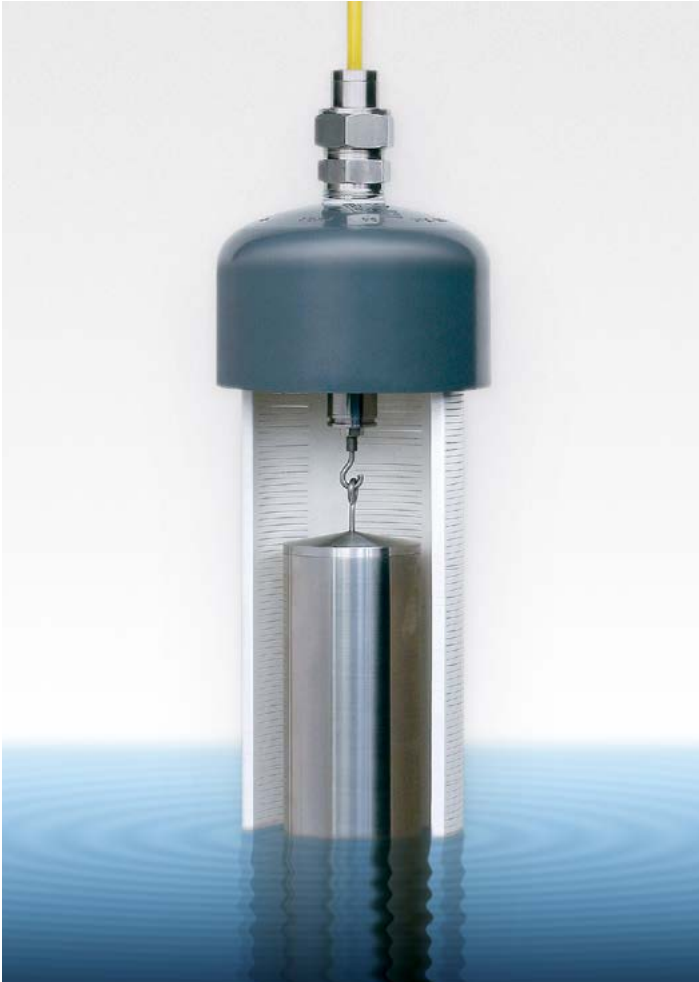
The Model 4675LV with cutaway revealing its internal components: a cylindrical weight suspended from the vibrating wire force transducer.
