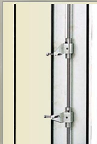
High deformation extensometer
