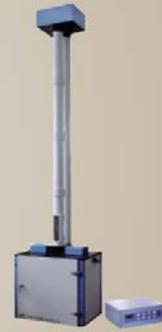
LC-300B falling arrow impact testing machine
