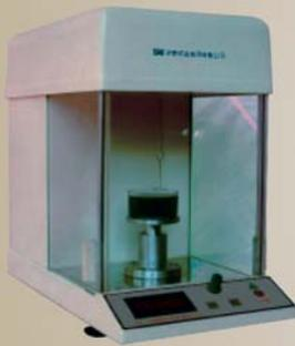
JZ-200A automatic liquid surface tonometer
