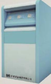
XGNB-W pipe explosive pressure testing machine
