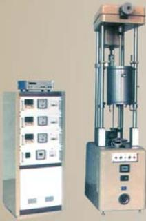
RDRC-1130 High temperature creep testing machine
