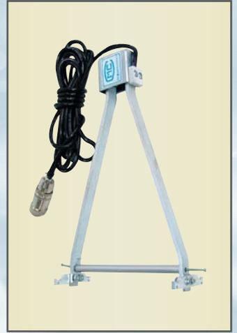
Small deformation extensometer
