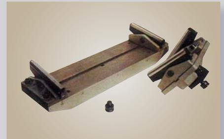
4-Points flexure test attachment
