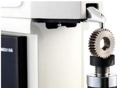
Gear hardness test
