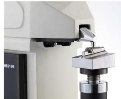
Hardness test of anchor clip
