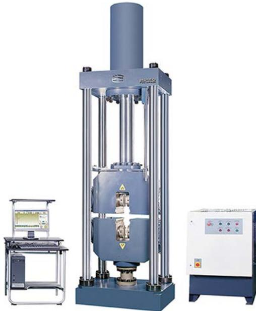
WAW- E Servo Hydraulic Tensile Testing Machine is mainly used for tensile test with high efficiency requirement. Equipped with relevant fixtures, this machine can also be used for compression, bending and shearing tests. Constant strain, Constant stress and constant displacement test are available. Strain velocity, stress velocity and displacement velocity conform to the requirement of GB, ASTM, DIN, ISO, JIS, BS etc. metal tensile testing standards.
