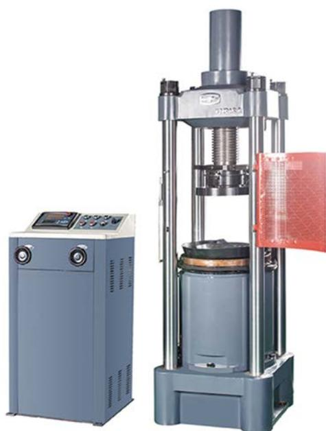
The series testing machine is mainly used to the compression test of concrete, cement and cement products, various blocks, hollow bricks, tiles and other ordinary building materials.
