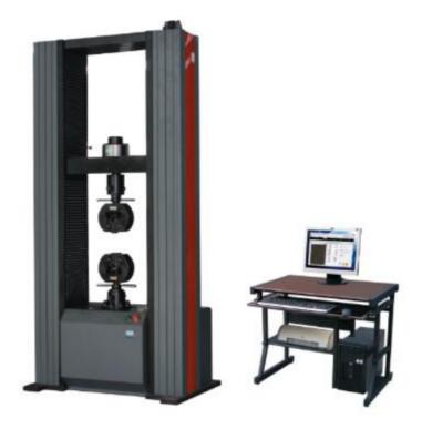
High strength light bar is used to fix the upper beam and the working table, so that it constitutes a high rigid structural frame.
